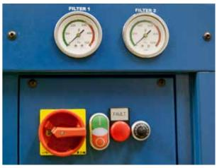
The FilterBench is equipped with pressure gauges clearly indicating when it is time to replace the filters.
